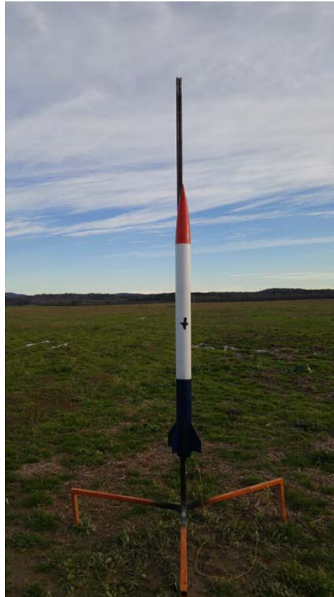
Figure 2. Subscale Launch Vehicle on the Launch Rail
